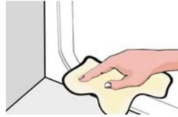
Clean surface with supplied alcohol wipe (MUST BE DRY)
