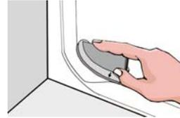
Without removing adhesive liner, place endcap LEVEL at the curb edge and inside the shower front.
