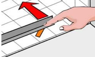
If adhesion is satisfactory, pull straight up and proceed with the installation. If not, surface preparation or mechanical attachment will be necessary.
